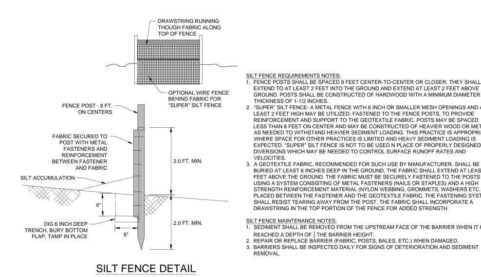
T FENCE REQUIREMENTS NOTES: FENCE POSTS SHALL BE SPACED 8 FEET CENTER-TO-CENTER OR CLOSER. THEY SHALL EXTEND TO AT LEAST 2 FEET INTO THE GROUND AND EXTEND AT LEAST 2 FEET ABOVE GROUND, POSTS SHALL BE CONSTRUCTED OF HARDWOOD WITH A MINIMUM DIAMETER THICKNESS OF 1-1/2 INCHES.
